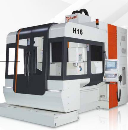
The swivel operation panel allows users to operate at any angle
